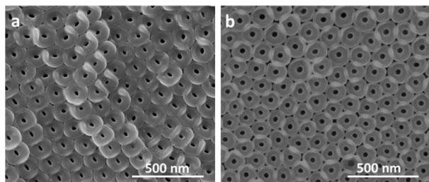
Figure 2. Nanotube pore size optimization. a) 15-25 nm and b) 35-45 nm inner diameter
