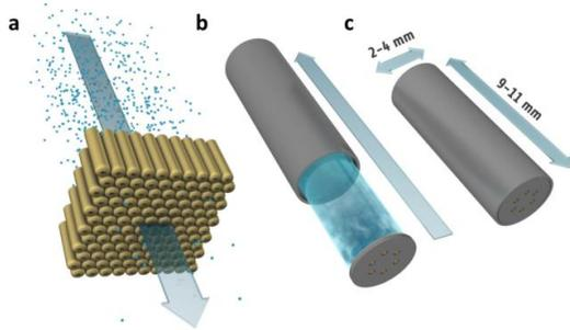
Figure 1. Schematic of nanotube membrane delivery device. a) Vertically aligned nanotube membrane controls flow of molecules. b) Membranes are combined with a reservoir device and loaded. c) Overview of full device.
