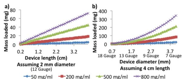
Figure 3. Filling capacity for different devices. a) Thin, 2 mm device, with length varying from 0.2 cm to 4 cm. b) Long, 4 cm device, with diameter varying from 0.7 to 4 mm. On both, concentrations from 50 mg/ml to 800 mg/ml are plotted as different lines (◆ – 50 mg/ml, ■ – 200 mg/ml, ▲ – 500 mg/ml, × – 800 mg/ml).
